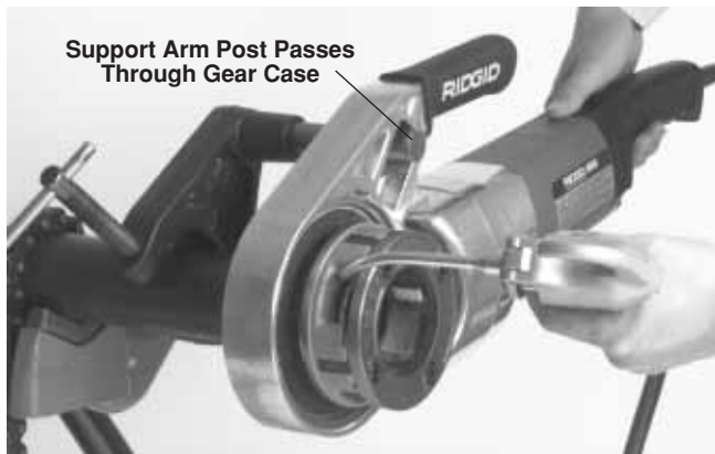
Figure 7 – Threading Pipe and Applying Oil
