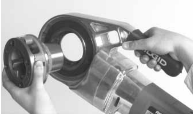
Figure 3 – Installing No. 11-R Die Heads
