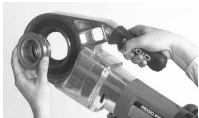
Figure 2 – Installation of 11-R Die Head Adapter
