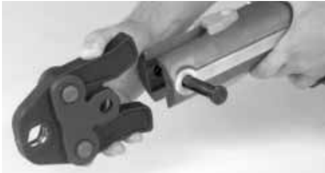
Figure 3 – Sliding Jaw Set Into CT400
