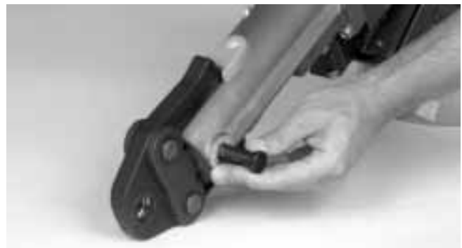
Figure 2 – Pulling The Jaw Set Mounting Pin Out
