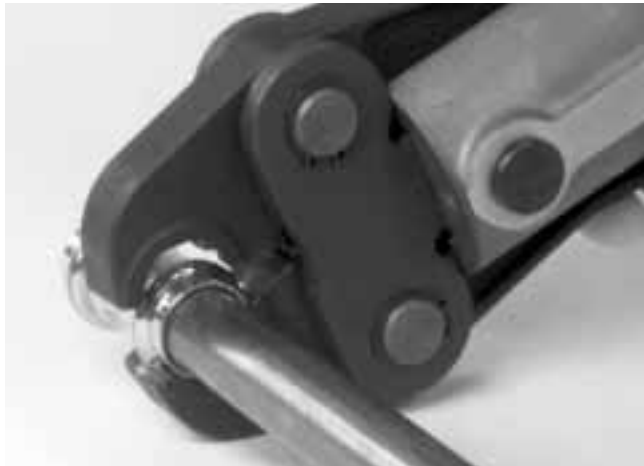
Figure 5 – Placing Scissor-Style Jaw Set Around Fitting
