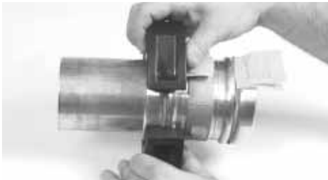
Figure 8 – Installing Press Ring Onto Fitting
