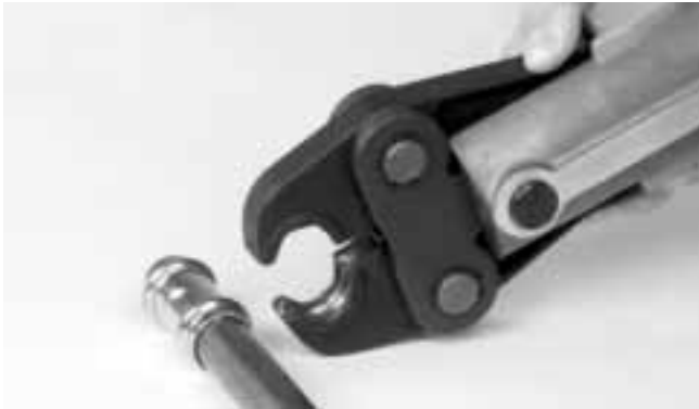
Figure 4 – Opening The Scissor-Style Jaw Set
