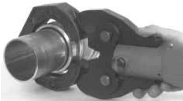
Figure 9 – Attaching Ring Actuator To Press Ring
