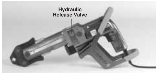
Figure 7 – Using Hydraulic Release Valve Button (If Needed)
