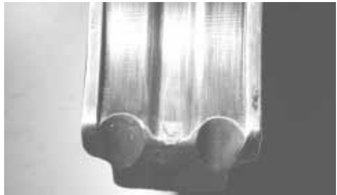
Figure 10 – Fitting Material Build-Up Requiring Cleaning
