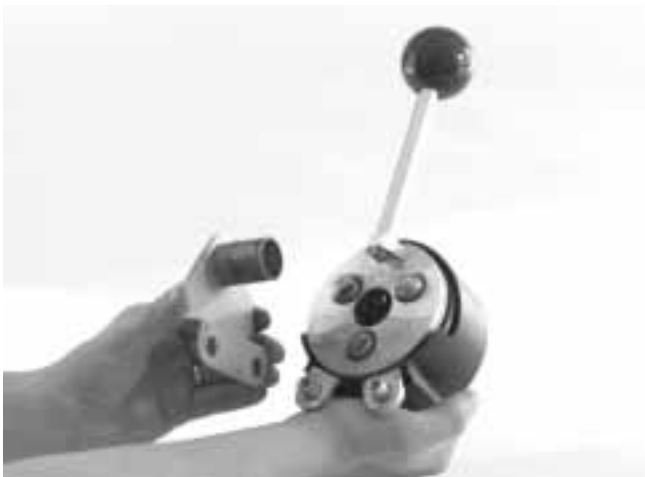
Figure 2 – Placing Mounting Bracket Into Auto Feed
