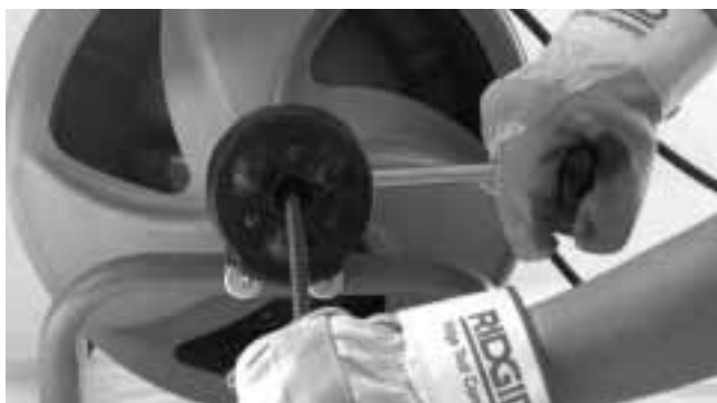
Figure 8 – Autofeed in Reverse Position
