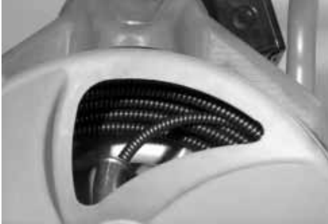
Figure 9 – Coil Cable Into Drum As Shown
