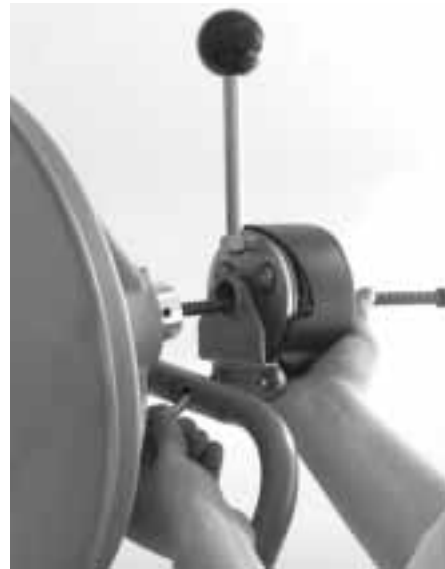
Figure 3 – Mounting Auto Feed Onto The Frame
