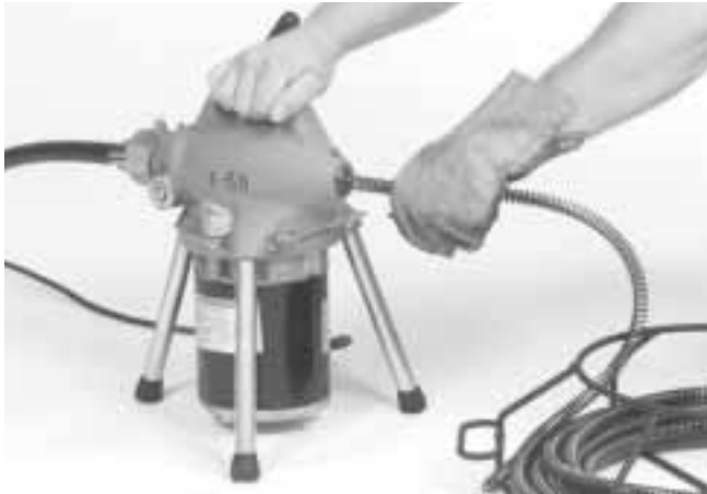
Figure 3 – Inserting Cable Into Front Of Machine
