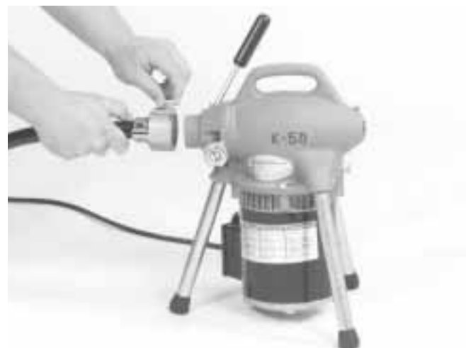
Figure 2 – Rear Guide Hose Attachment
